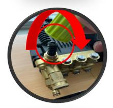
Place the lime adjustment knob back on top of the spring and tighten in a clockwise motion until the knob can't turn anymore.
