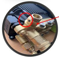
Undo the fastening screw (highlighted) with an allen key (size 2.0) to allow the adjustment ring to be lowered.
